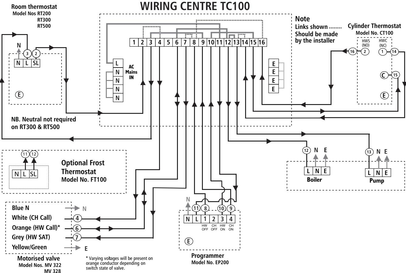
Note: links shown on diagram should be made by the installer.
