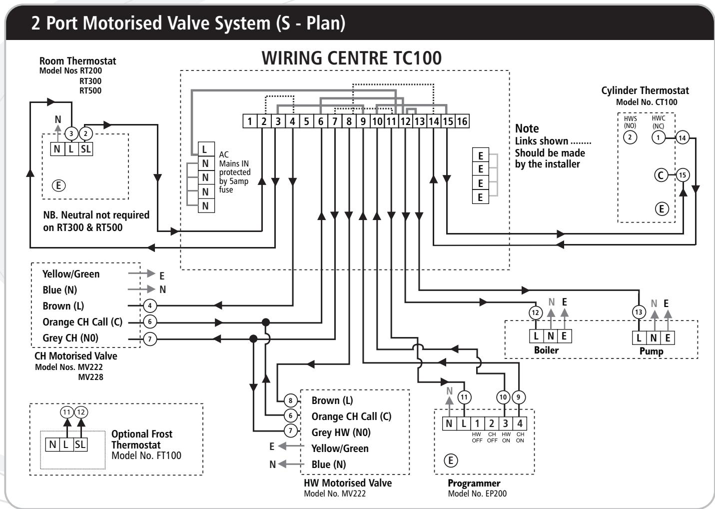
Note: links shown on diagram should be made by the installer.
